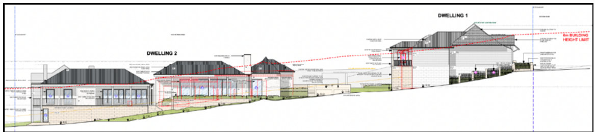
Figure 1: Western elevation showing the contravention being the new construction above the red dashed line.
